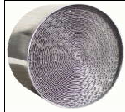
Fig. 2. Close-up view of PFT filter substrate showing the alternating tapered trapezoidal ducts and filtration media
