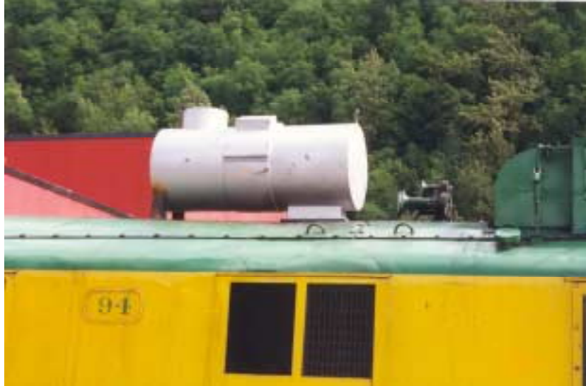
Figure 2 – DCL Catalytic Converter Installed on Locomotive
