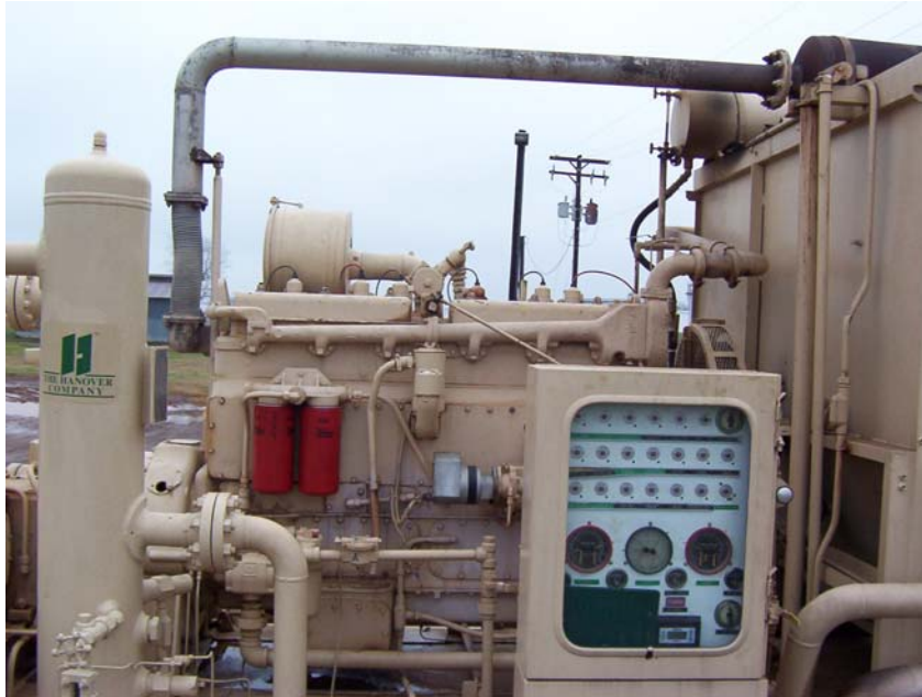
Figure 2-3. Small, uncontrolled, rich-burn compressor engine (Northeast Texas).
