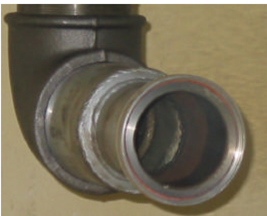
(c): The pipe terminal that was fastened to the high volume PM sampler
