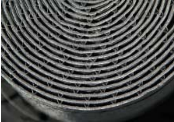
Figure 2: Close-up view of PFT substrate showing the alternating tapered trapezoidal ducts and filtration media
